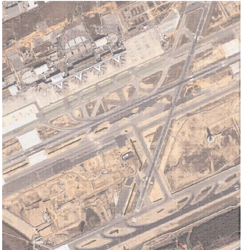
Figure 2: When Barcelona Airport built a new runway (07R/25L) no fewer than eight new runway incursion opportunities were created
